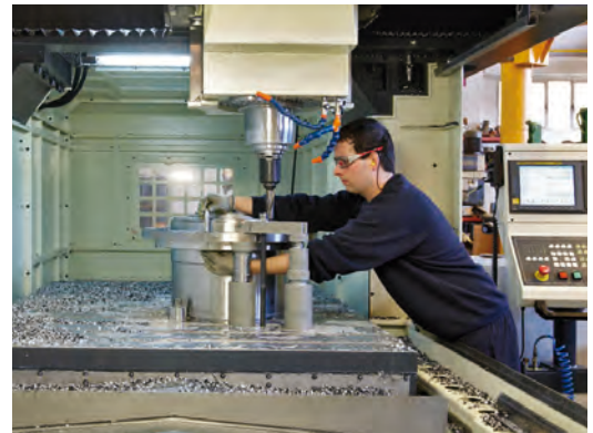
Machining of barrel coupling's hub.
