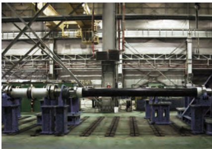
Carbon Fibre Shaft combined with LAMIDISC® coupling.
