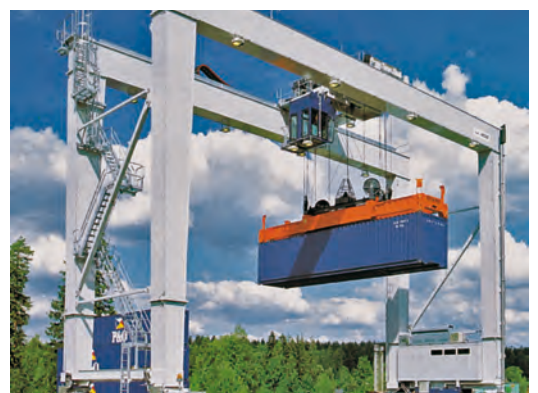
Rubber tyred Gantry crane.
